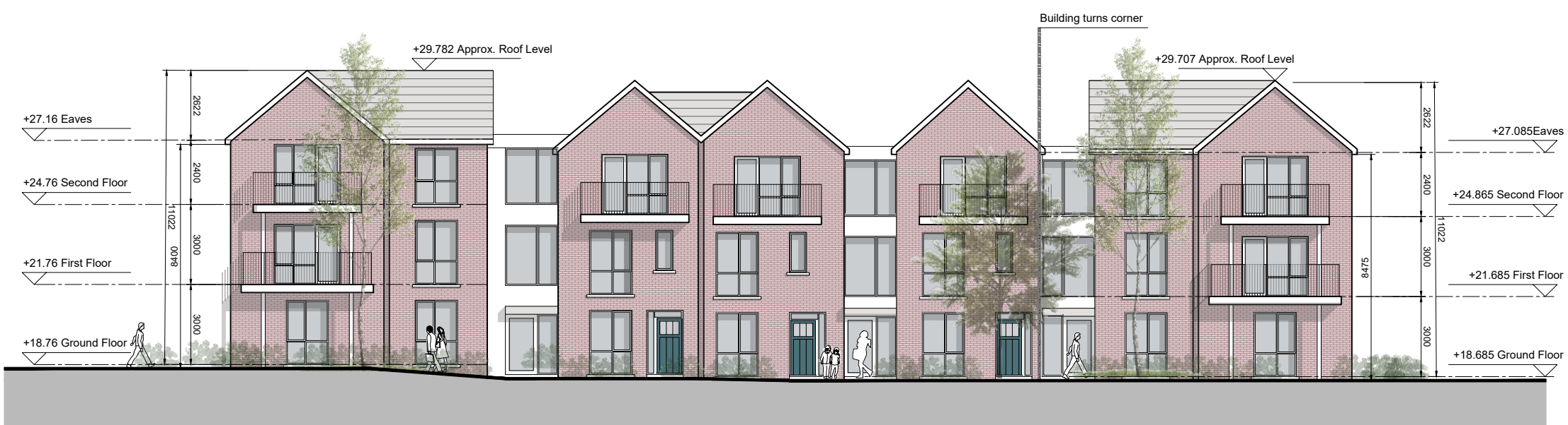
DUPLEX BLOCK A EAST ELEVATION (STREET ELEVATION)
